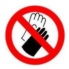
Gloves must not be worn when using this machine.
